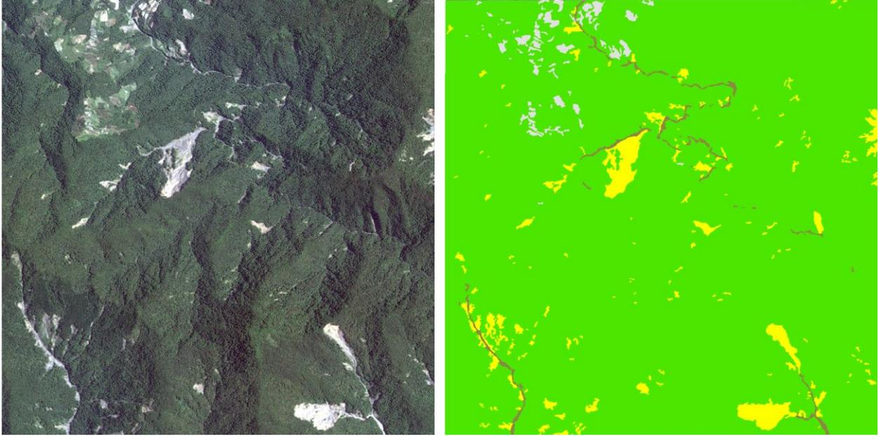
**Figure 1 Samples for Formosat 2 imagery and the corresponding land cover mapping. (Green: vegetation, Yellow: landslide, Brown: riverbed, Gray: miscellaneous)**
