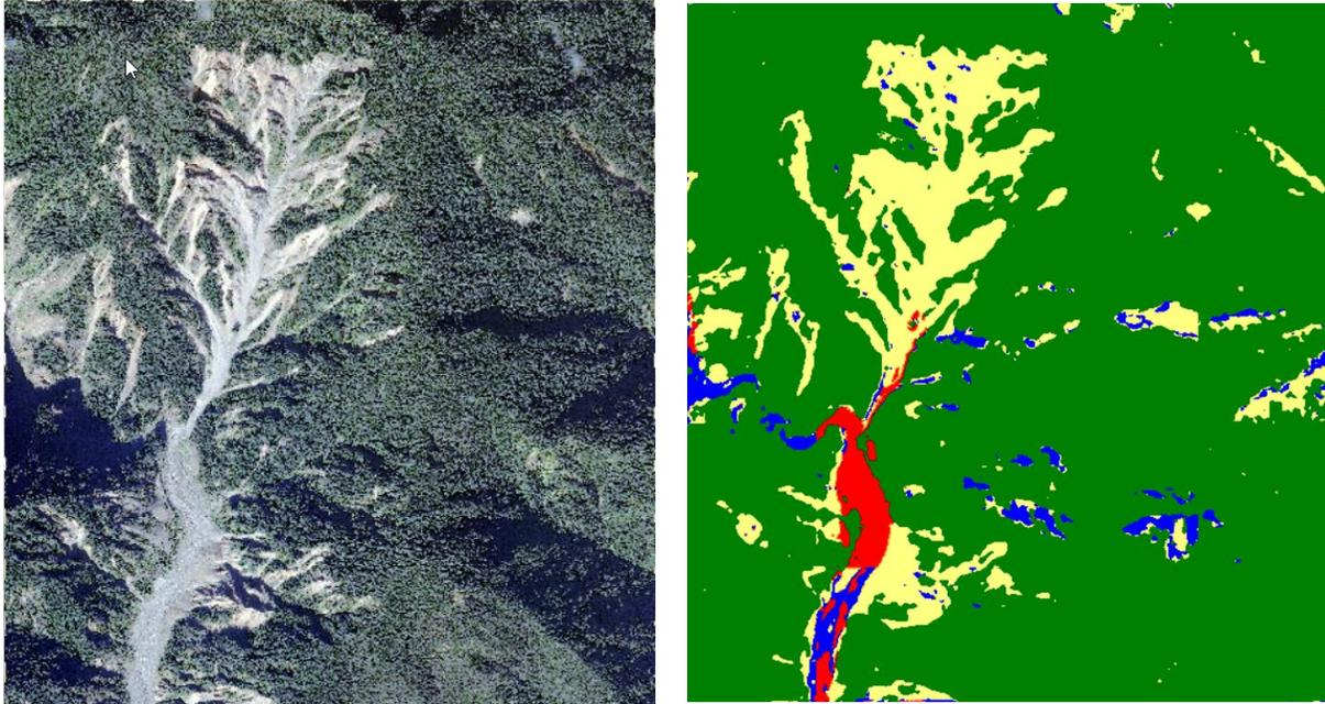
**Figure 6 Classification results of Kompsat-3. (Dark Green: vegetation, Light Green: landslide, Red: riverbed, Blue: Water, Magenta: Miscellaneous)**
