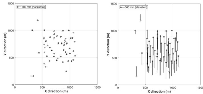
Figure 8. The difference vectors of horizontal coordinates (left) and elevations (right) on all check points (Case 4-2)
