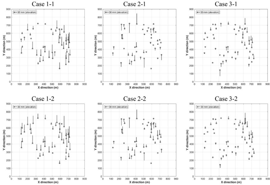
Figure 5. Vectors of elevation differences on all check points
