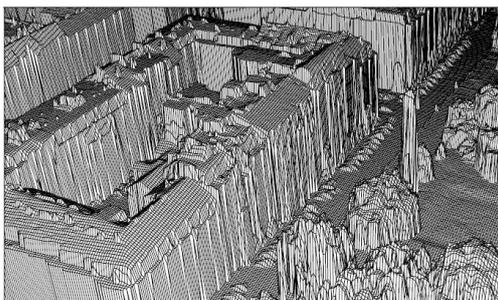
Figure 4. Using LiDAR to construct DSM
