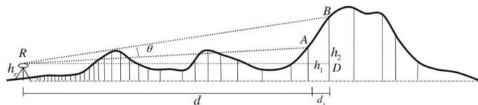
Figure 2. Varied intervals resulting from the adaptive sampling algorithm (Han & Li., 2010) Han & Juan (2016) use image as the source of analysis data for terrain obscuration. It uses the image extraction edge to obtain the masked edge line of each position, as shown in Figure 3. The image extraction method result is much faster than the conventional DSM method in speed, which can also improve the calculation effectively.
