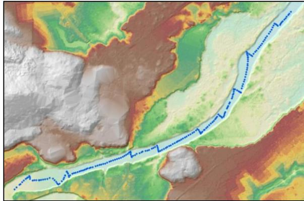
Figure 1. The bathymetric points superimposed to the DTM
