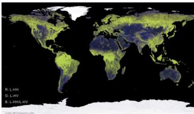
ALOS PALSAR-2 global mosaic at 25 m (0.8 arcsec) pixel spacing. HH+HV polarisation composite.
