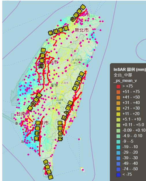
Figure 3. Ground changing rate map of Taiwan calculated from 4-years of descending Sentinel-1 data.
