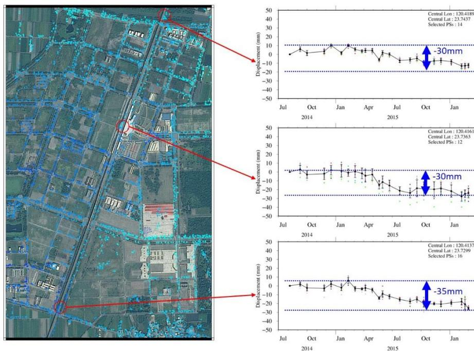
Figure 5. Time series of displacement at Yunlin high-speed rail station and at both ends along the railway.
