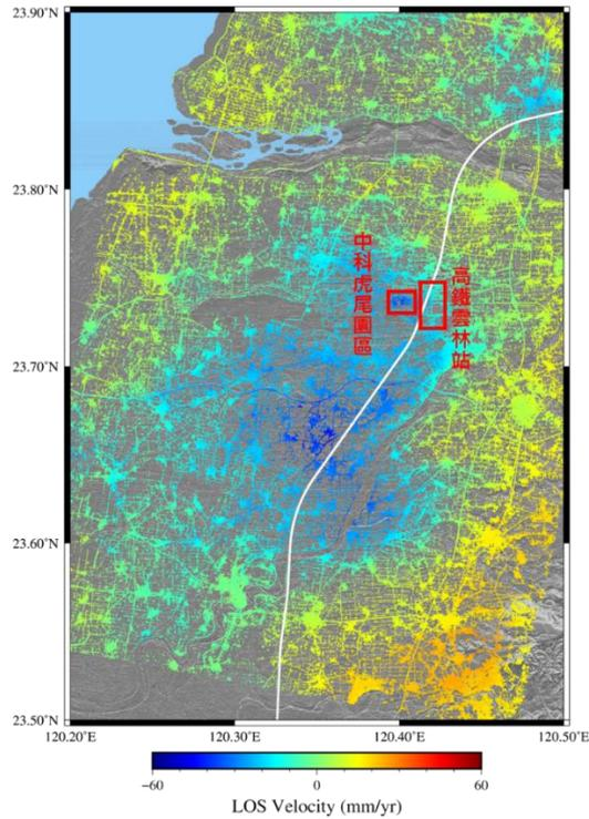
Figure 4. The velocity map in line of sight on Yunlin high-speed railway. (White line is high-speed railway and red squares are Central Taiwan Science Park at Huwei and high-speed rail station)
