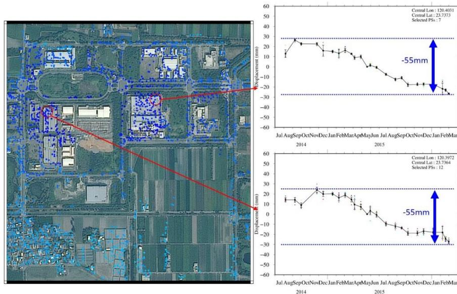
Figure 6. Time series of displacement in Central Taiwan Science Park at Huwei
