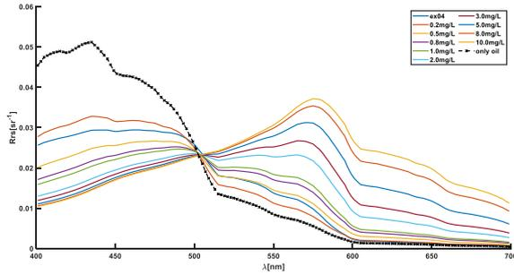
Figure 6 Remote sensing reflectivity of A4 site (low petroleum concentration) with suspended sediment concentration
