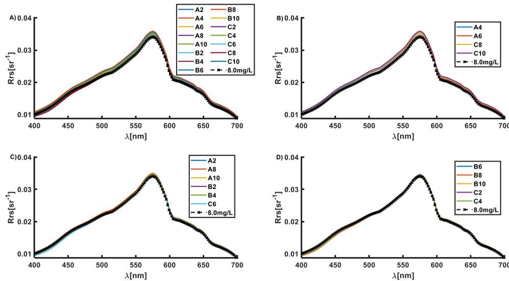
Figure 11 Remote sensing reflectance of suspended sediment concentration at 8.0mg/L varying with petroleum concentration. A) remote sensing reflectance of each site. B) remote sensing reflectance of low petroleum concentration. C) remote sensing reflectance of petroleum concentration. D) remote sensing reflectivity of high petroleum concentration
