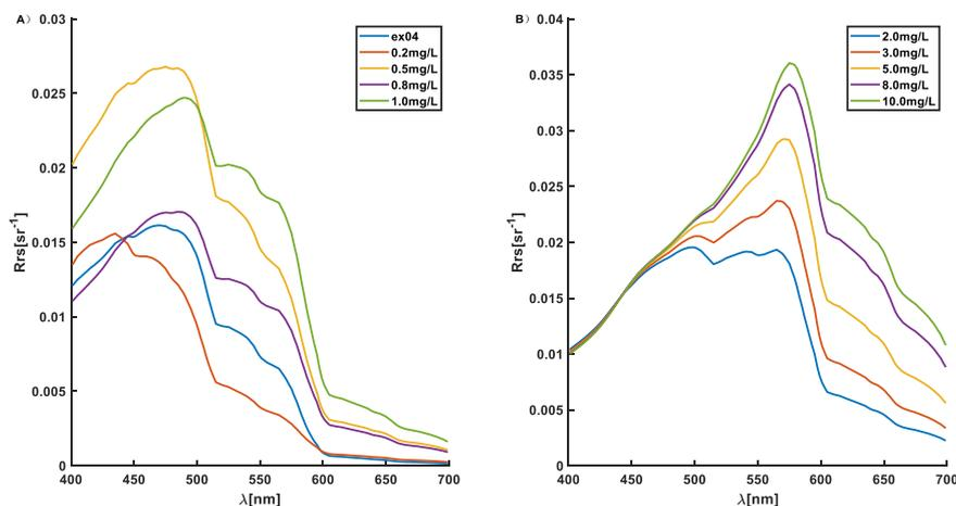
Figure 5 Remote sensing reflectance of suspended sediment at different concentrations. A) remote sensing reflectance image of suspended sediment concentration at 1 mg/L; B) remote sensing reflectance image of suspended sediment concentration at 2-10 mg/L.
