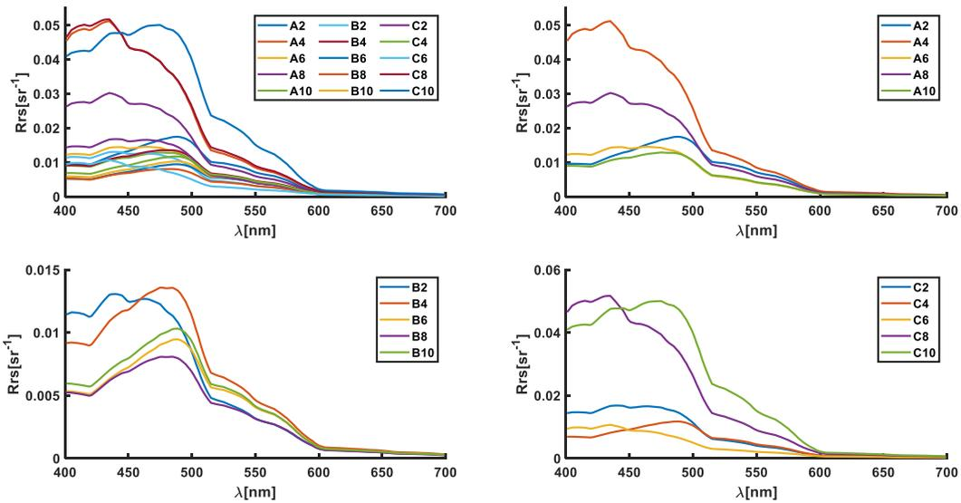
Figure 2 The remote sensing reflectance of each site calculated by Hydrolight. A) remote sensing reflectance of three site. B) remote sensing reflectance of site A. C) remote sensing reflectivity of site B. D) remote sensing reflectivity of site C
