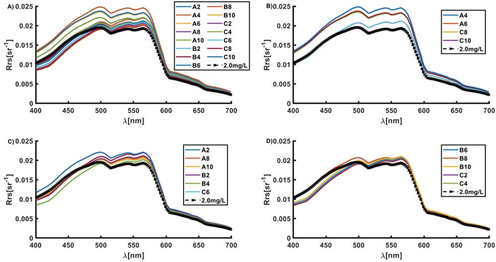
Figure 10 Remote sensing reflectance of suspended sediment concentration at 2.0mg/L varying with petroleum concentration. A) remote sensing reflectance of each site. B) remote sensing reflectance of low petroleum concentration. C) remote sensing reflectance of petroleum concentration. D) remote sensing reflectivity of high petroleum concentration
