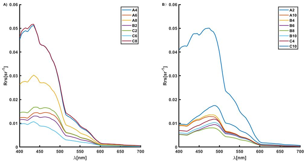
Figure 4 Remote sensing reflectance of two kinds of petroleum substances. A) the peak value of remote sensing reflectance for petroleum substances is between 430 and 440 nm; B) the peak value of remote sensing reflectance for petroleum substances is between 480 and 490 nm.
