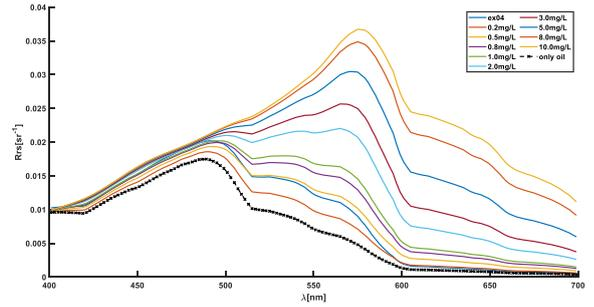
Figure 7 Remote sensing reflectivity of A2 site (middle petroleum concentration) with suspended sediment concentration
