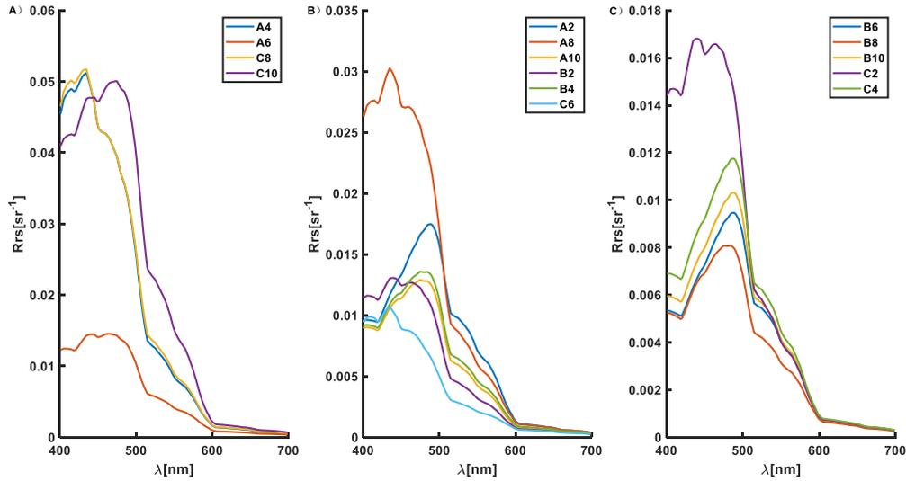
Figure 3 Remote sensing reflectance of petroleum in different average concentration  $\lambda$  ranges. A) the remote sensing reflectance curve of water with low petroleum; B) the remote sensing reflectance curve of water with middle petroleum; C) the remote sensing reflectance curve of water with high petroleum
