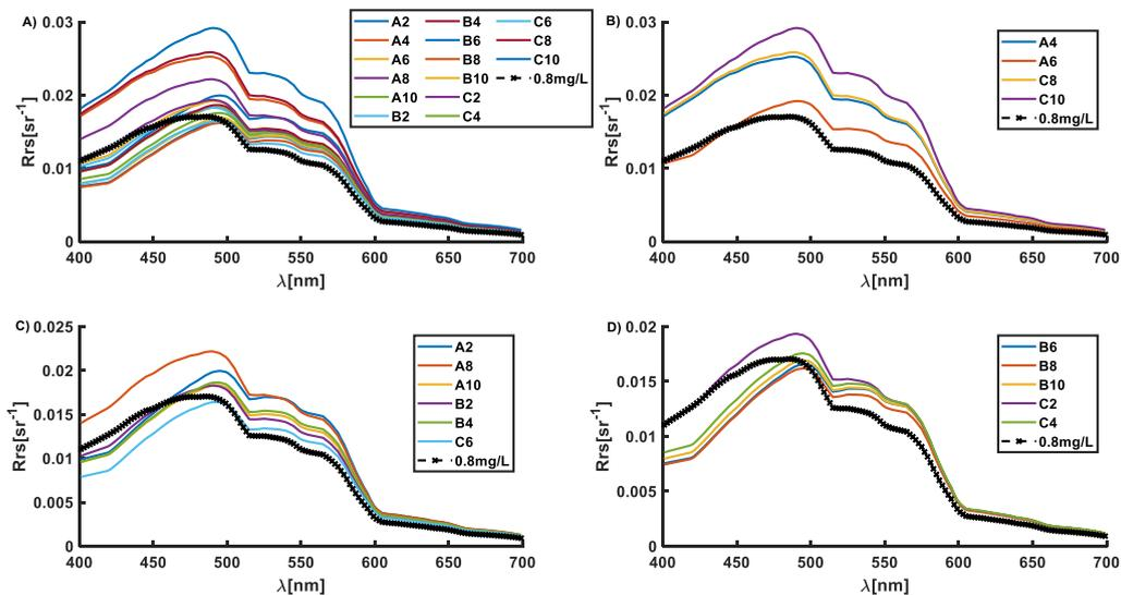
Figure 9 Remote sensing reflectance of suspended sediment concentration at 0.8mg/L varying with petroleum concentration. The black dotted line is the remote sensing reflectance only containing suspended sediment. A) remote sensing reflectance of each site. B) remote sensing reflectance of low petroleum concentration. C) remote sensing reflectance of petroleum concentration. D) remote sensing reflectivity of high petroleum concentration
