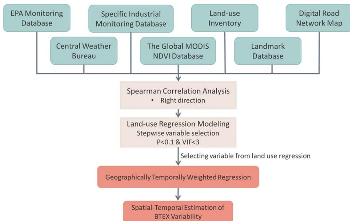
Figure 2. Framework of spatial modelling of BTEX pollutants distribution using GTWR.
