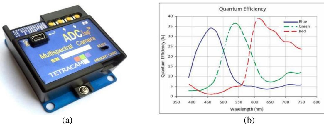
**Figure 1.** (a) ADC Micro multispectral camera (Tetracam, Inc., CA, USA) and (b) spectral response characteristics of the camera for blue that is blocked for NIR sensing, green, and red, employed in this study ([www.tetracam.com](http://www.tetracam.com)).
