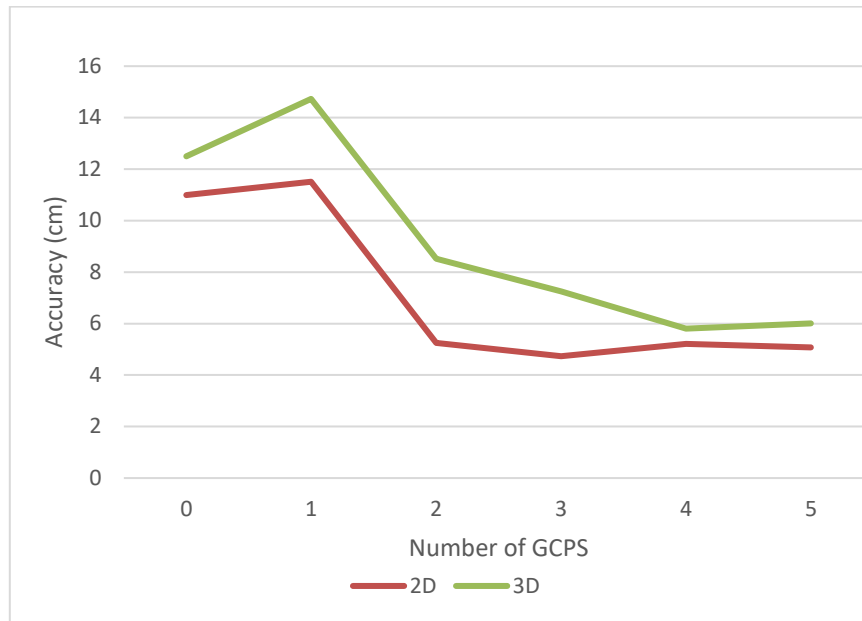
Figure 7: Accuracy variation of the RTK drone
