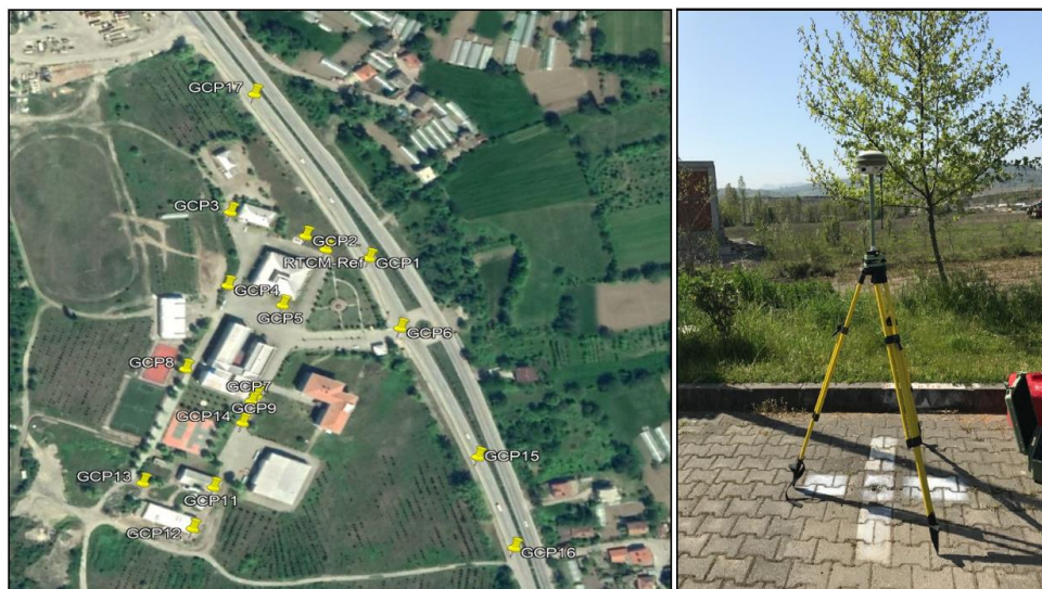
Figure 3. The location of established GCPs and an instance GNSS measurement
