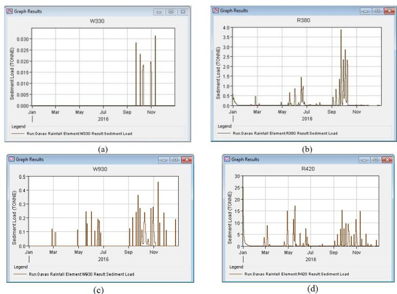
**Fig. 5.** Simulated sediment yield in Pilan Watershed (a) sub-basin W330 and (b) reach R380 and in Matiao Watershed (c) sub-basin W930 and (d) reach R420.
