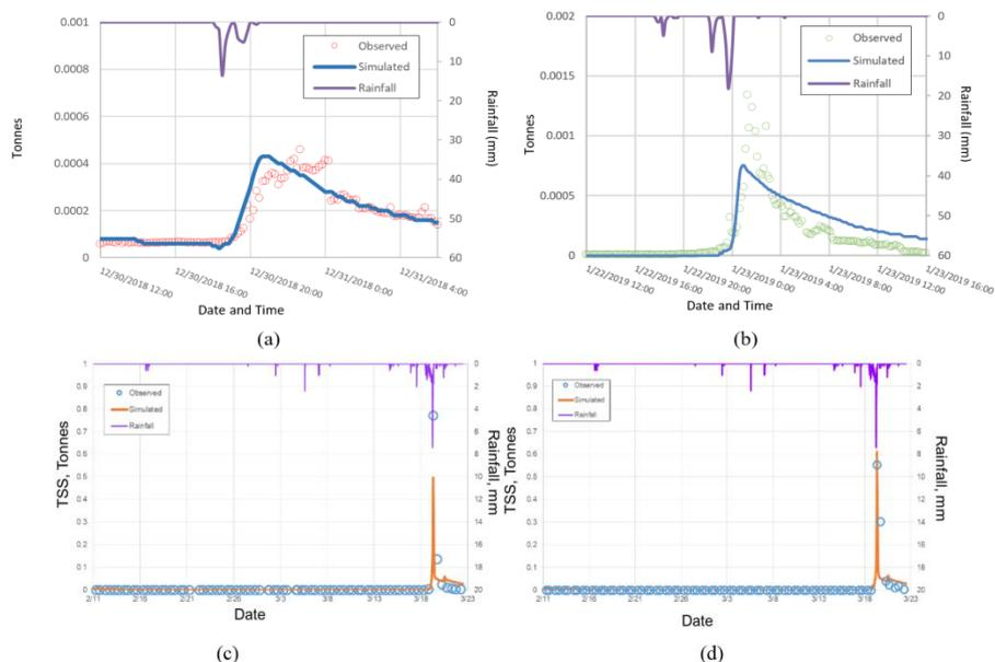
**Fig. 4.** Graphs of the HEC-HMS MUSLE sediment model simulated sediment yield and observed TSS during (a) calibration and (b) validation of Pilan Watershed sediment model, and calibration of Matiao Watershed sediment model at (c) Matiao and (d) Binugsayan Bridge.
