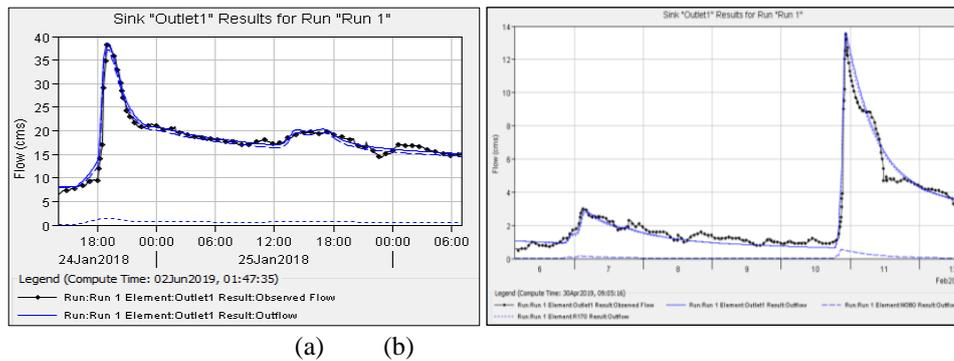
**Fig. 3.** Comparison of the simulated river discharge versus the field-surveyed discharge data of the (a) Matiao River from January 24 to 26, 2018 and (b) Pilan River on February 6- 12, 2018.
