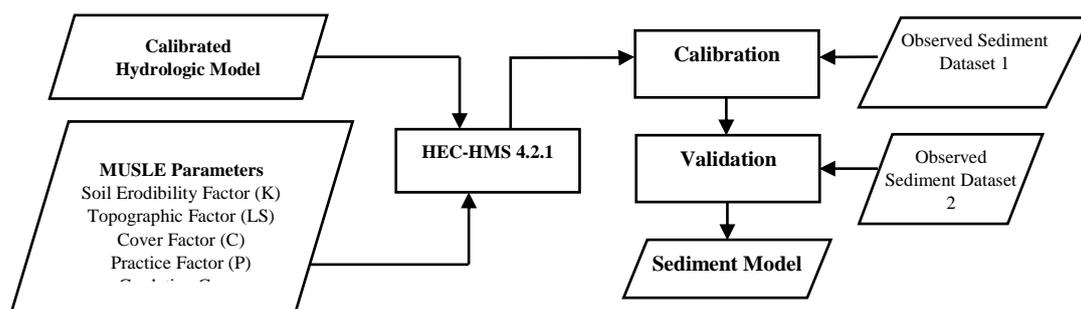
**Figure 2.** Level 0 of the data flow diagram for the sedimentation modeling using HEC-HMS.
