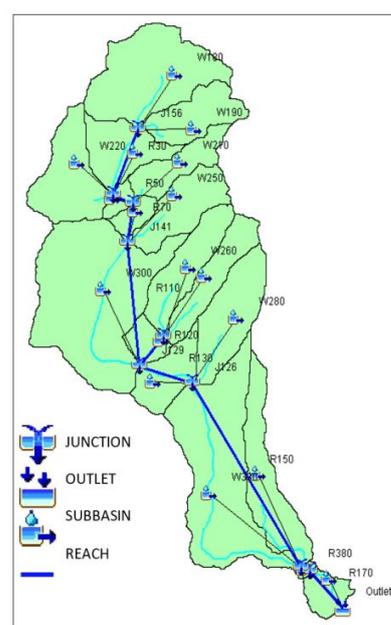
b. Pilan Hydrologic Model
