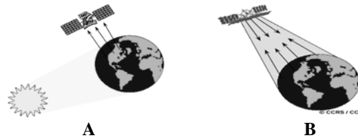
Figure 1. Remote sensing systems: (a) passive remote sensing system and (b) active remote sensing system. (source: www.rfwireless-world.com)
