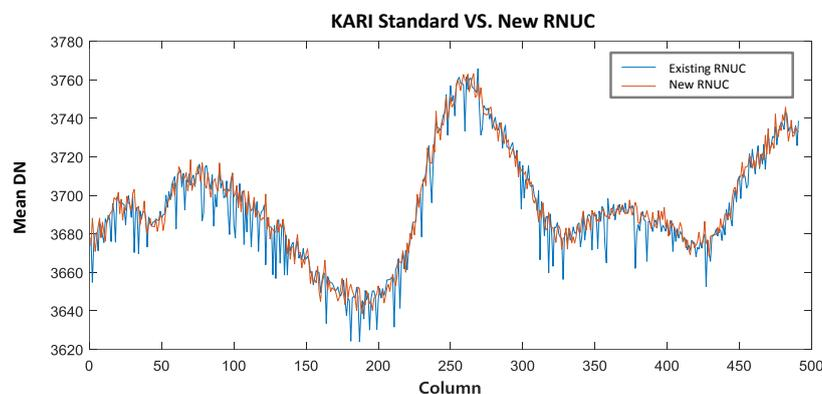
Figure 5. Comparison of Result of Existing RNUC and New RNUC
