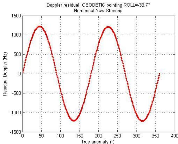
**Figure 3. Residual Doppler vs. true anomaly after yaw steering**
