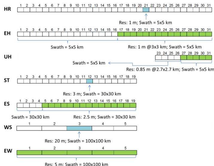
Figure 1. KOMPSAT-5 basic and enhanced operation mode
