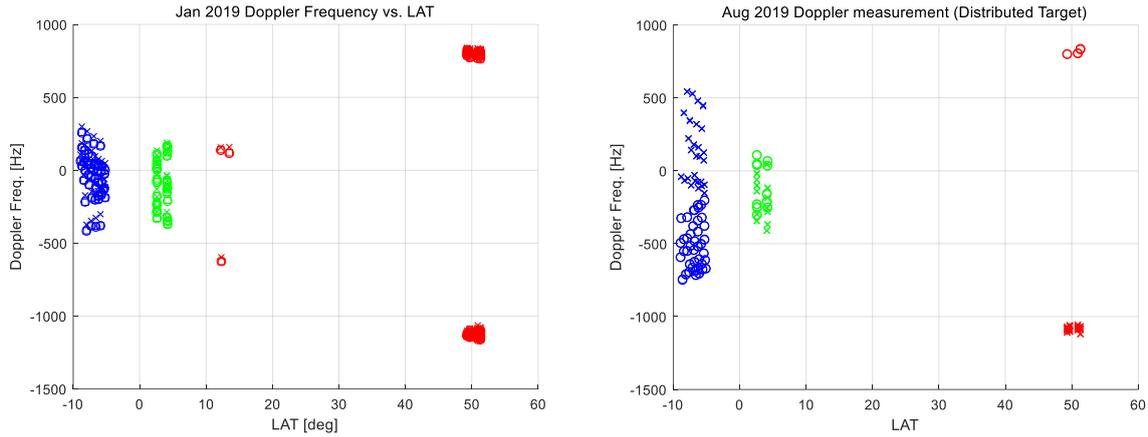
**Figure 4. Residual Doppler measured from January(left) and August(right) image**
