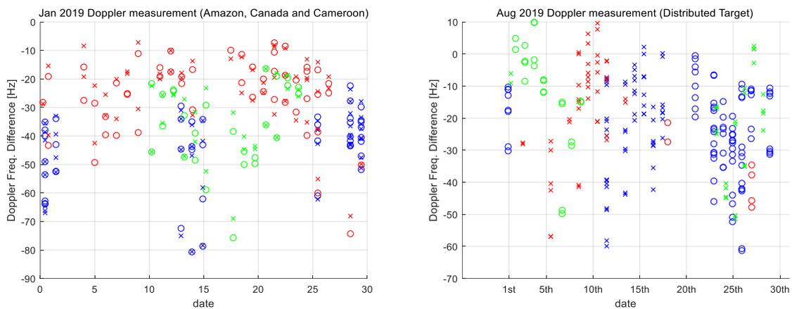
**Figure 5. Doppler centroid difference measured from ancillary and echo signal**
