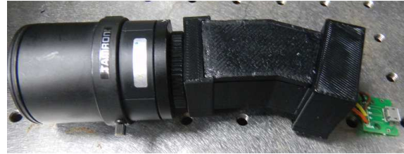
Figure 1. 110g lightweight hyperspectral imager with lens, the imager was 50g and the fore lens was 60g.
