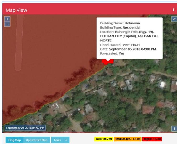
Figure 8. Point-and-click assessment of impacts of a forecasted flooding to a structure.
