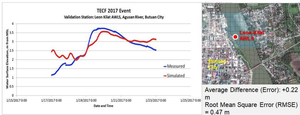
Figure 10. Example simulated water surface elevation/level (WL) for flooding condition.
