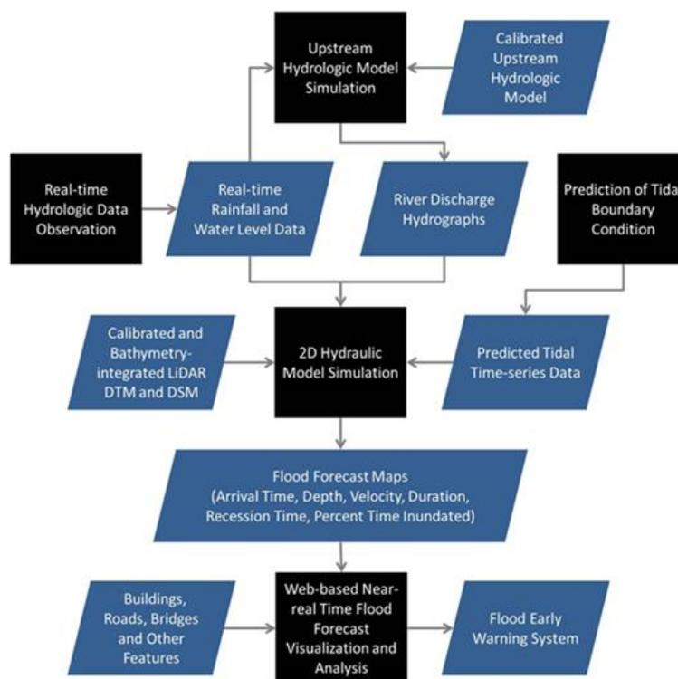
Figure 2. Flowchart of developing the near-real time flood event visualization and damage estimations (Source: Makinano-Santillan and Santillan, 2016).
