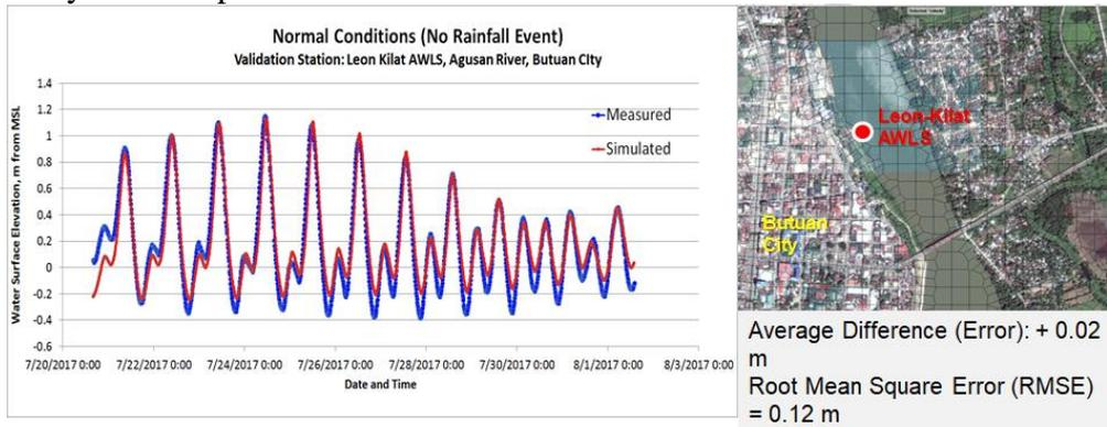
Figure 9. Example simulated water surface elevation/level (WL) for “normal” or non-flooding condition. The simulated levels were compared with data recorded by a WL sensor.
