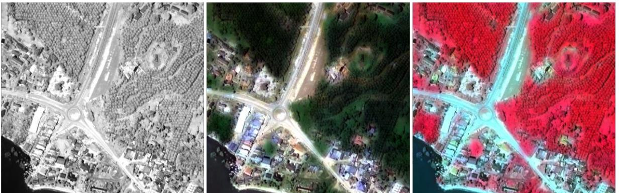
Figure 3. Results of pan-sharpening using our simple algorithm: Effective intensity (left), true color image (middle) and false color (RGB=NIR,Red,Green) image (right).
