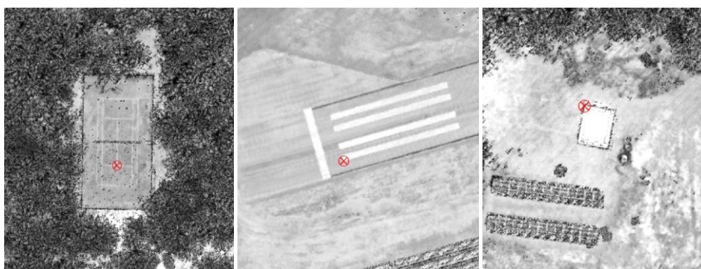
Figure 5. Selected examples of checkpoints measured on interpolated intensity images resampled from Lidar point clouds at 10cm.
