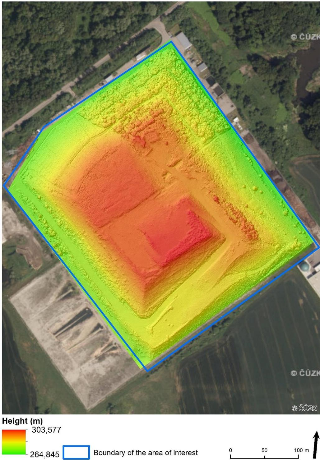
Figure 3 DSM from UAV
