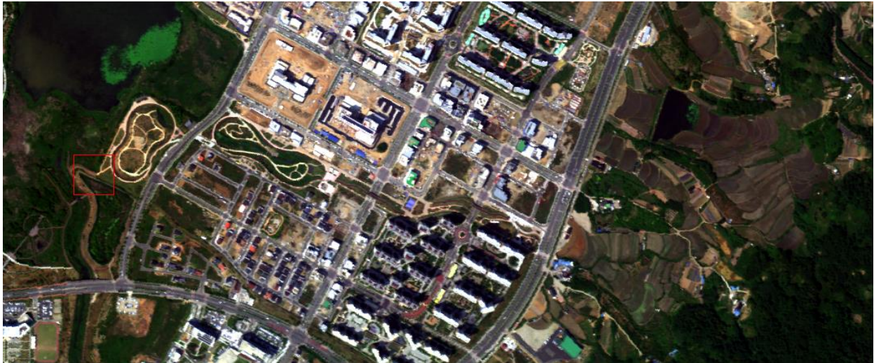
Figure 2. RGB color composite of study area. The study area was chosen Jeonju city and image was acquired by AISA FENIX hyperspectral sensor
