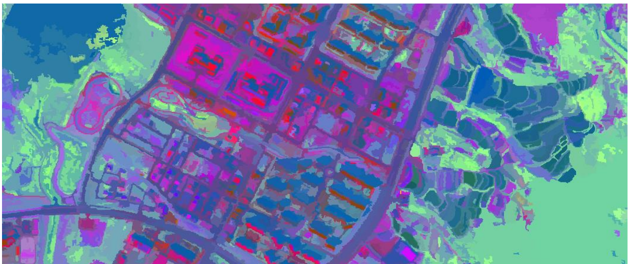
Figure 5. The result of MRS method, object mean value color composite of PC 1, 2 and 3 bands
