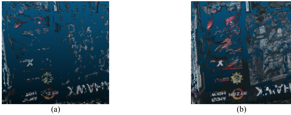
Figure 7. Point clouds of a plane (a) by the traditional method; (b) through the proposed strategy
