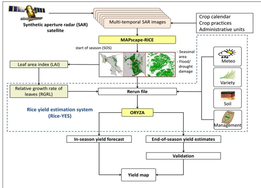
Figure 2. Process diagram of yield estimates using SAR and ORYZA crop growth model.
