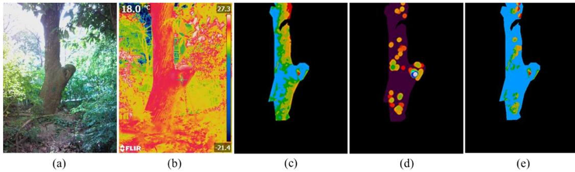
Figure 8. Images of Defect Tree *Cinnamomum Camphora* (a) True Colour Image; (b) Thermal Image; (c) K-means Clustering; (d) Sobel Gradient Filter; (e) Final Detection Map
