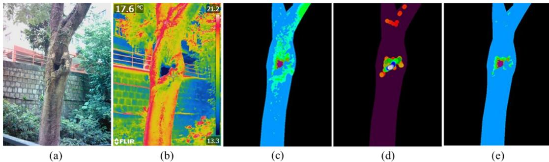
Figure 6. Images of Defect Tree *Delonix Regia* (a) True Colour Image; (b) Thermal Image; (c) K-means Clustering; (d) Sobel Gradient Filter; (e) Final Detection Map
