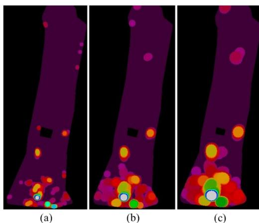
Figure 4. Results of Thermal Images after Applying Sobel Gradient Filter, Feature Scaling and Maximum Pooling (a) Disk Size = 5, Gradient Threshold = 0.1; (b) Disk Size = 9, Gradient Threshold = 0.1; and (c) Disk Size = 13, Gradient Threshold = 0.1
