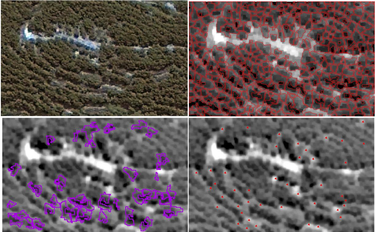
**Figure 3: Individual Tree Delineation Steps For A Subset Image Of The Study Site (Plot 1): (A) Pleiades Of High-Resolution Images; (B) Morphology Strategic And Marker-Controlled Watershed Segmentation, Where Segmented Crowns Are Represented In Red (C) The Geometric Shift Reflects The Aggregated Proportion Crown Of Detected Trees; (D) Number Of Standing Dead Tree (Shown In The Red Triangle)**
