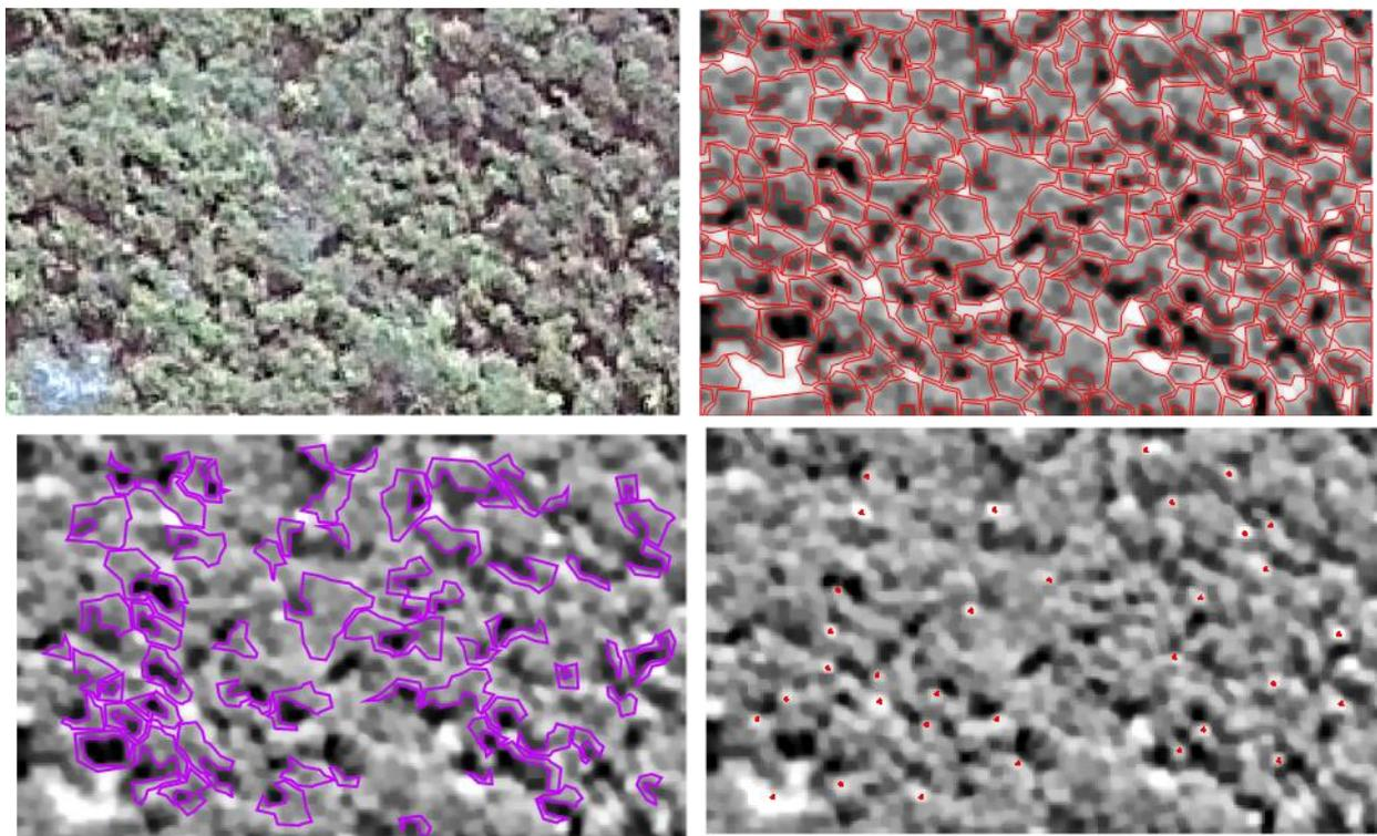
**Figure 5: Individual Tree Delineation Steps For A Subset Image Of The Study Site (Plot 3): (A) Pleiades Of High-Resolution Images; (B) Morphology Strategic And Marker-Controlled Watershed Segmentation, Where Segmented Crowns Are Represented In Red (C) The Geometric Shift Reflects The Aggregated Proportion Crown Of Detected Trees; (D) Number Of Standing Dead Tree (Shown In The Red Triangle)**
