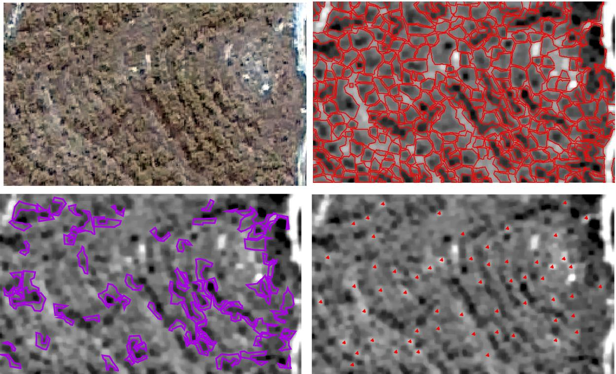
**Figure 4: Individual Tree Delineation Steps For A Subset Image Of The Study Site (Plot 2): (A) Pleiades Of High Resolution Images; (B) Morphology Strategic And Marker-Controlled Watershed Segmentation, Where Segmented Crowns Are Represented In Red; (C) The Geometric Shift Reflects The Aggregated Proportion Crown Of Detected Trees; (D) Number Of Standing Dead Tree (Shown In The Red Triangle)**
