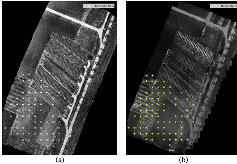
**Figure 5:** Extracted MPs after outlier removal: (a) reference image, (b) subject image.
