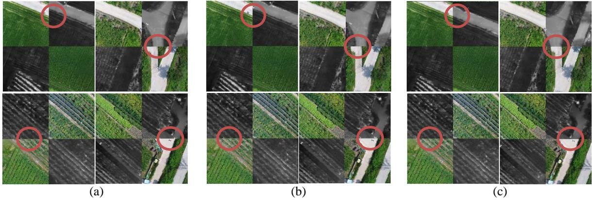
**Figure 6:** Mosaic images of automatic co-registration result: (a) raw image (b) phase correlation (c) proposed method.
