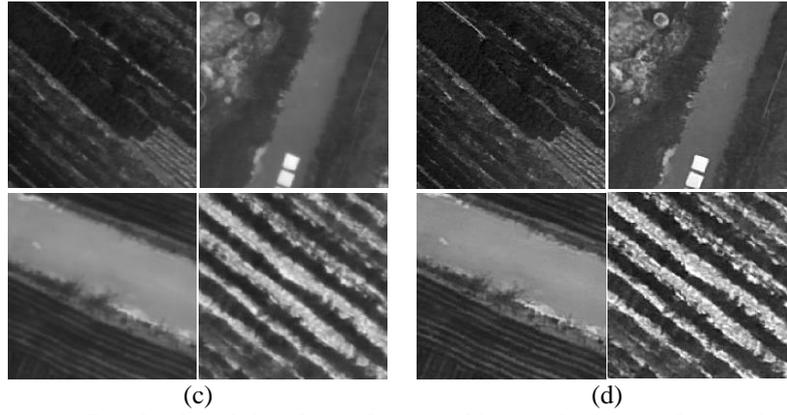
**Figure 4:** Result of applying the unsharp masking method: (a) reference image, (b) reference image with edge enhanced, (c) subject image, and (d) subject image with edge enhanced.
